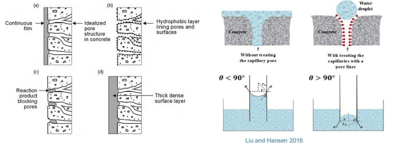
Schematic representation of the different types of surface treatment of concrete:
