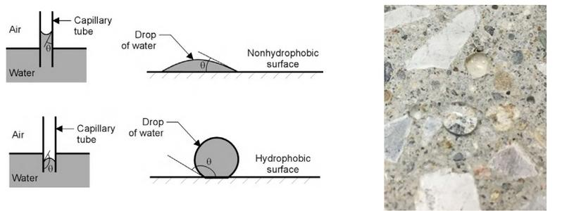
Interaction between water and a nonhydrophobic or hydrophobic material; illustrated for a capillary (left) and a concrete surface (right).
