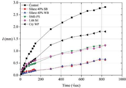
Fig. 2—Absorption results for initial penetrating sealer products for full-coverage application.
