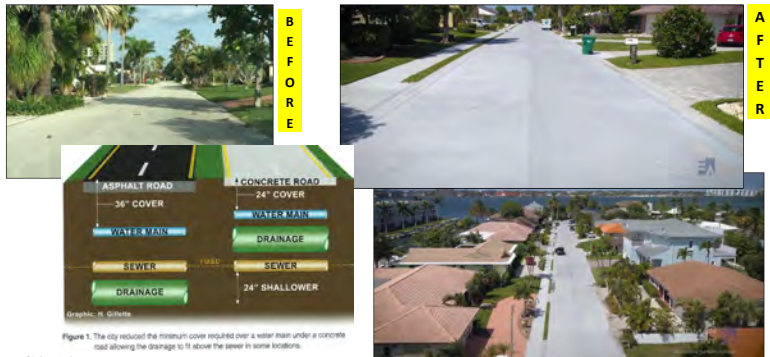
Figure 1. The city reduced the minimum cover required over a sewer main under a concrete road allowing the drainage to fit above the sewer in some locations.
