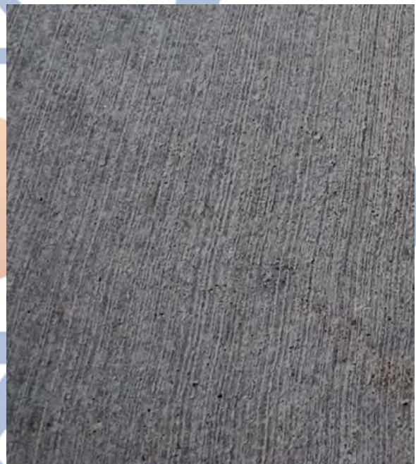
Nano Silica Mix with Little to No Surface Abrasive Wear
