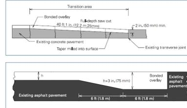
Figure 72. Mill and fill transition for concrete overlay of concrete pavement (adapted from ACPA 1998)
