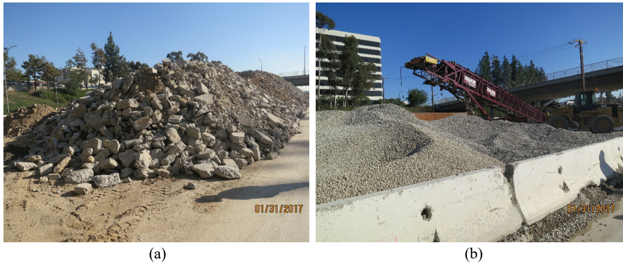
Figure 5. Rubble from old concrete pavement (left) and processed recycled concrete aggregate (right).
