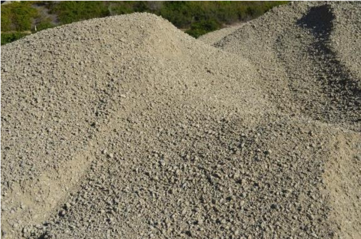
Photo A-24. Stockpile of recycled concrete aggregate produced on-site.
