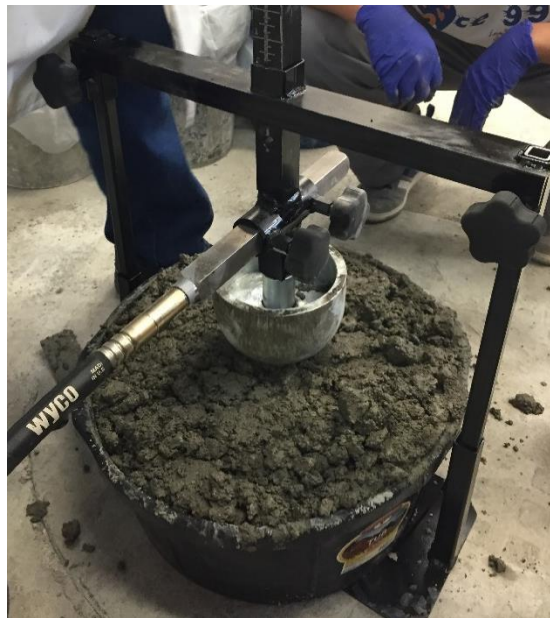
Figure 1- Depth of Penetration under Static Load
