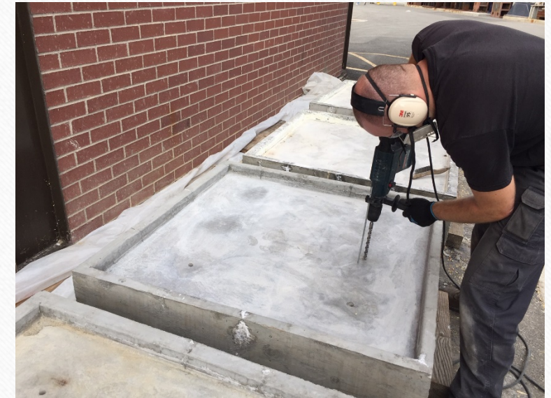
Taking concrete powder samples
