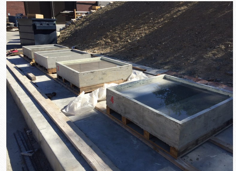
Pouring salt water on the slabs
