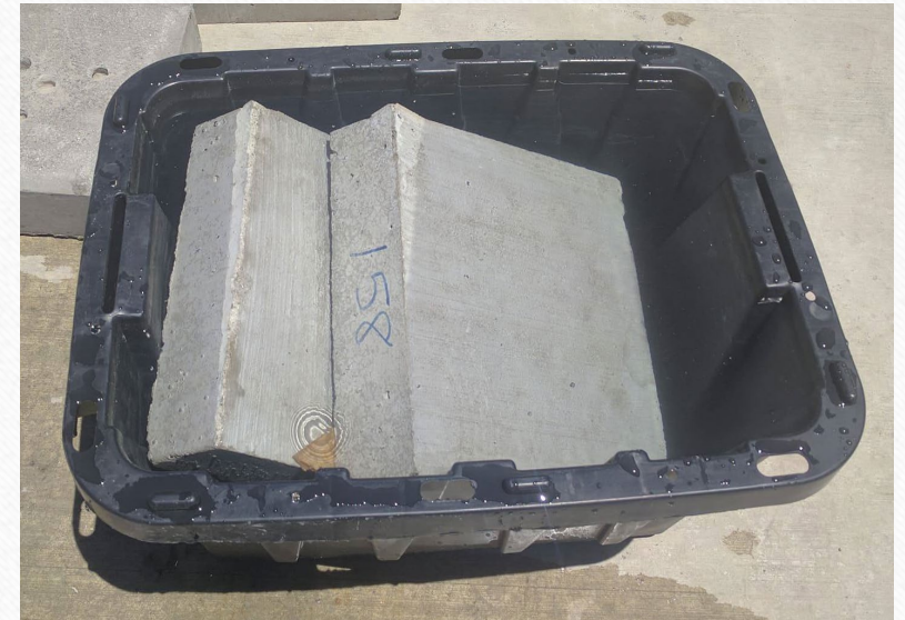
Two specimens were immersed in sodium chloride solution
