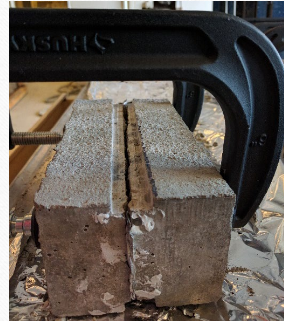
Formation of required crack width
