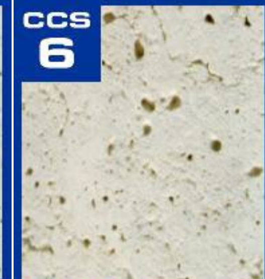
CCS 6 Applied Film Thickness 0.005 inches
