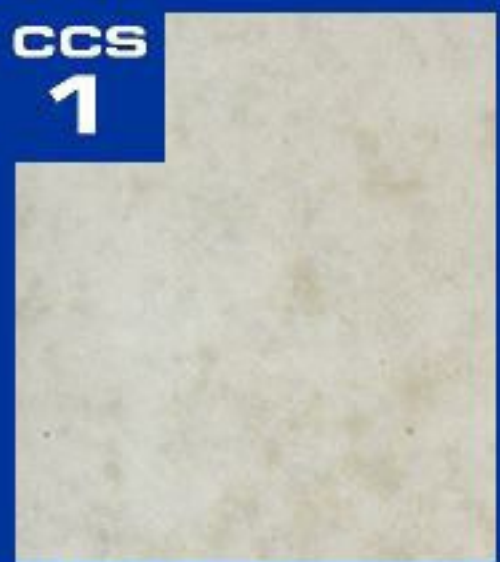
CCS 1 Applied Film Thickness <0.0005 inches
