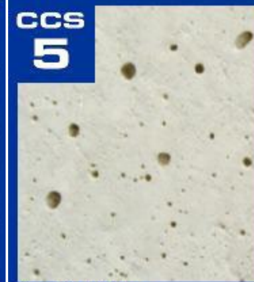
CCS 5 Applied Film Thickness 0.004 inches
