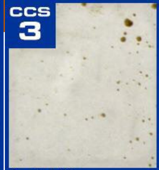
CCS 3 Applied Film Thickness 0.002 inches
