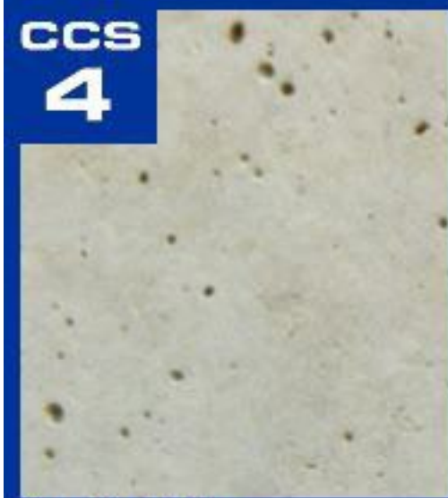
CCS 4 Applied Film Thickness 0.003 inches
