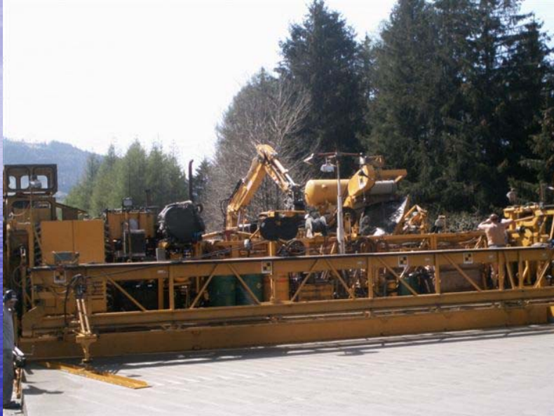
Paver with longitudinal smoother
