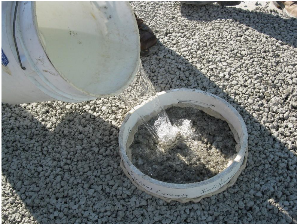
Pervious concrete surface infiltration
