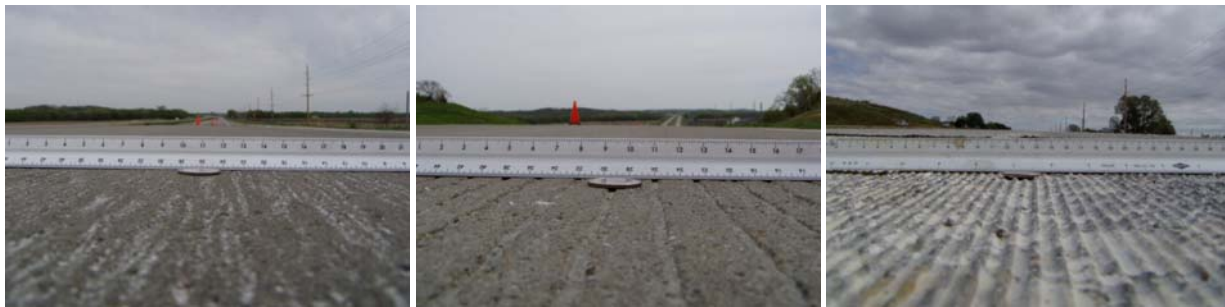
Figure B-1. Photographs of typical drag, tining, and diamond grinding textures.
