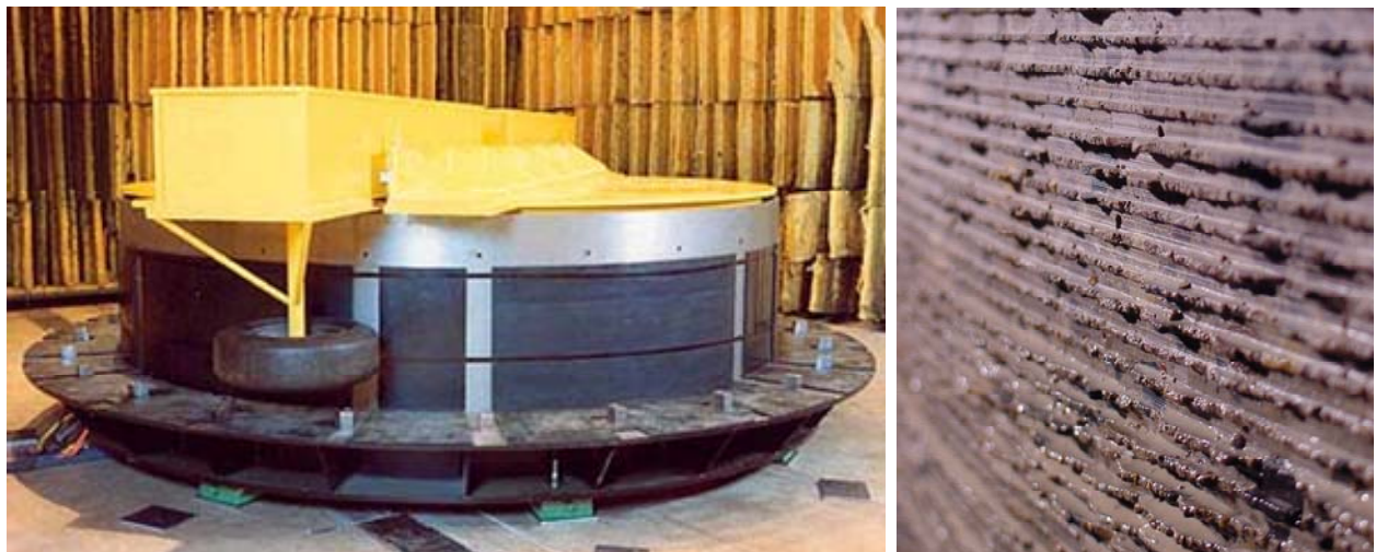
Figure 23. TPTA test equipment and sample surface (source: Purdue SQDH).
