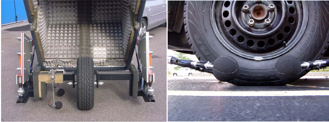
Figure 20. CPX and OBSI test equipment.
