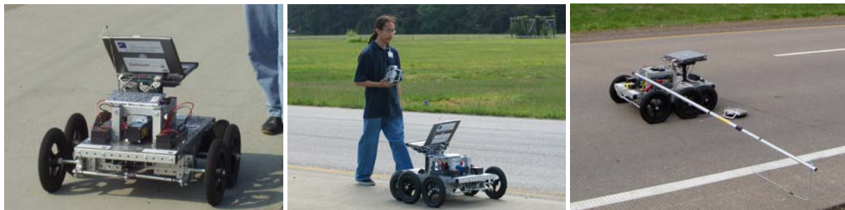
Figure B-2. Photographs of RoboTex measurement system.
