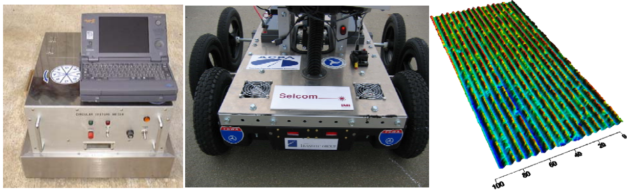
Figure 21. CTM and RoboTex test equipment (source: CP Tech Center).
