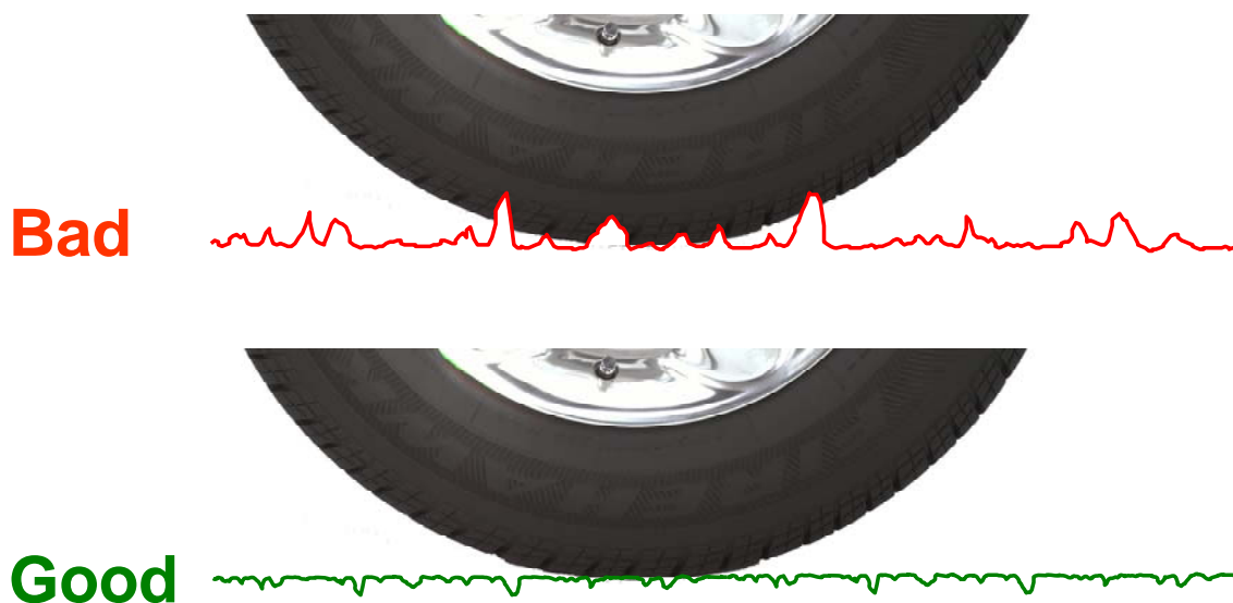
Figure 24. Conceptual schematics of “bad” and “good” texture.
