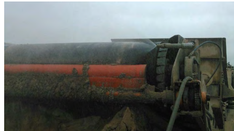
Example concrete crushing dust suppression system (photo: Duit Construction).
