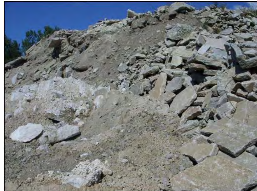
Stockpile of broken concrete with excessive fines
