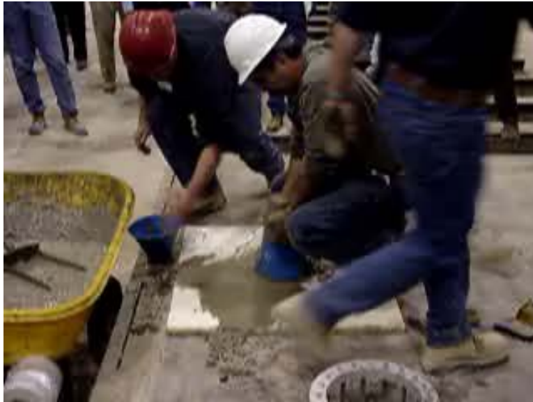
Slump flow test (ASTM C1611) Prestressed Engineering Corp, Blackstone, IL, USA
