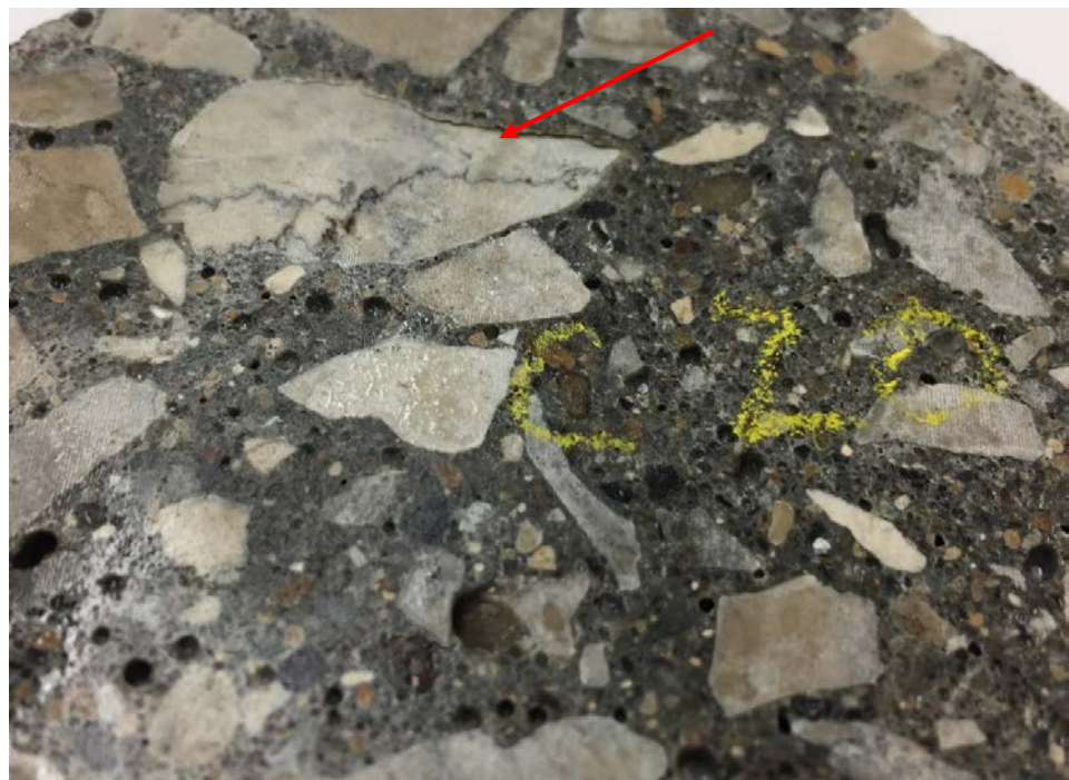
20% \text{CaCl}_2 @ 40°F for 28 days
