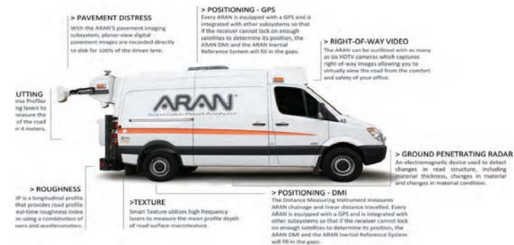
Fugro Roadware Automatic Road Analyzer (ARAN)
