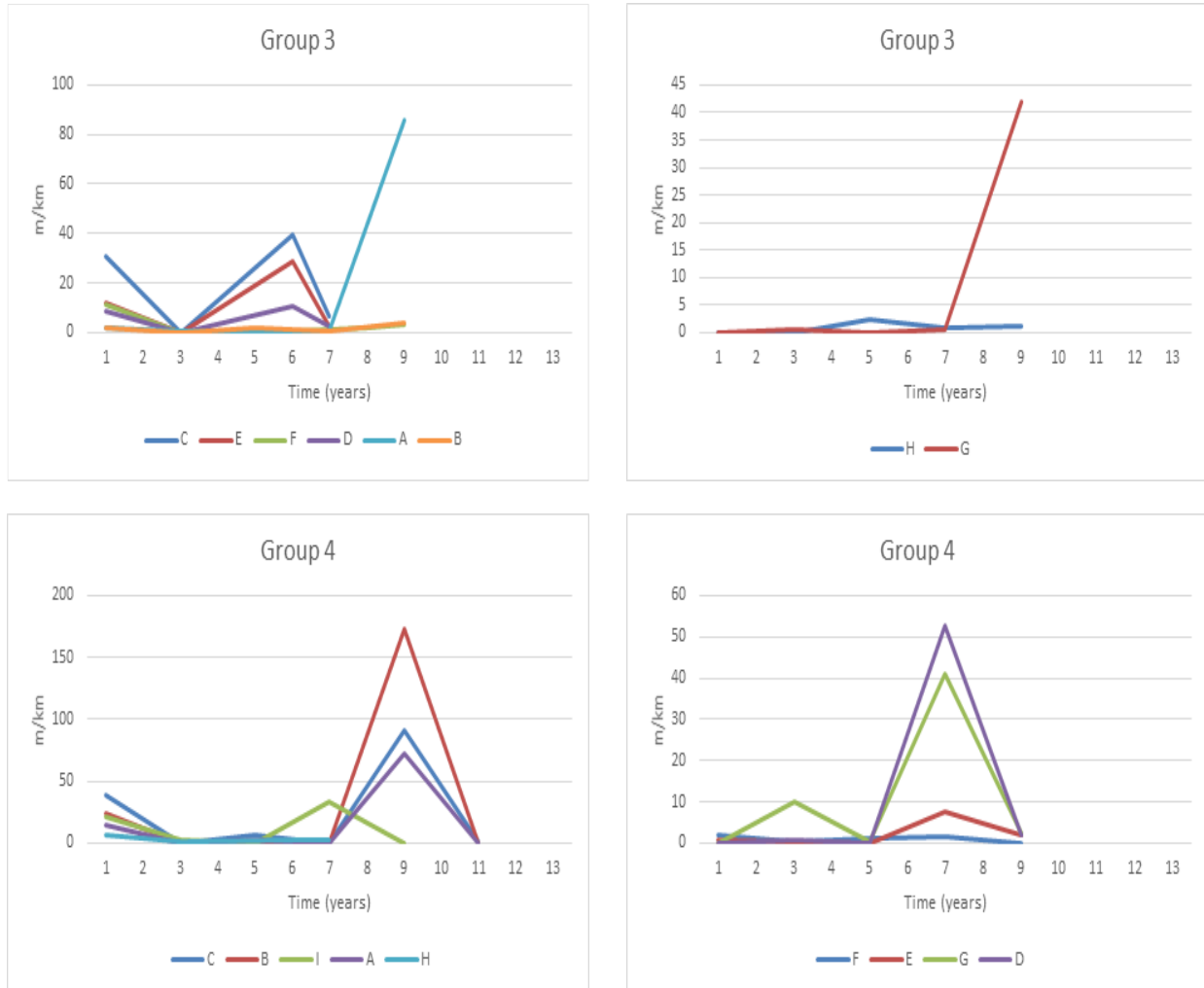
Figure 14. Moderate longitudinal cracking deterioration for Groups 3 and 4
