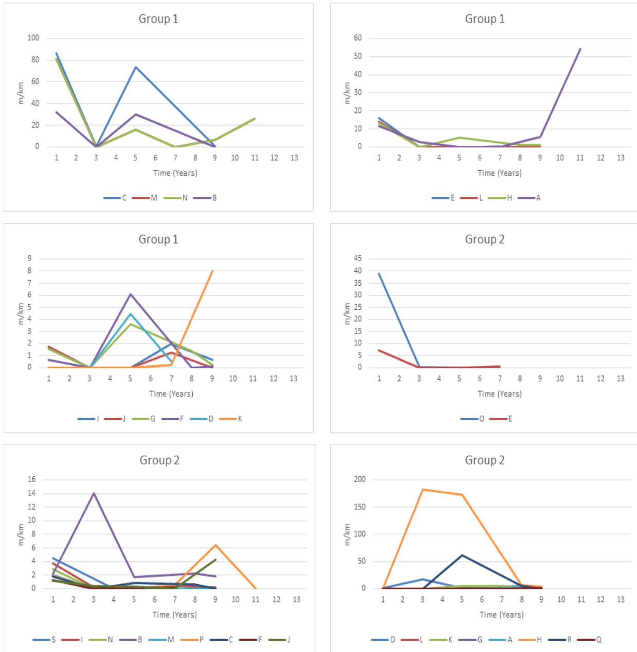
Figure 9. High transverse cracking deterioration for Groups 1 and 2
