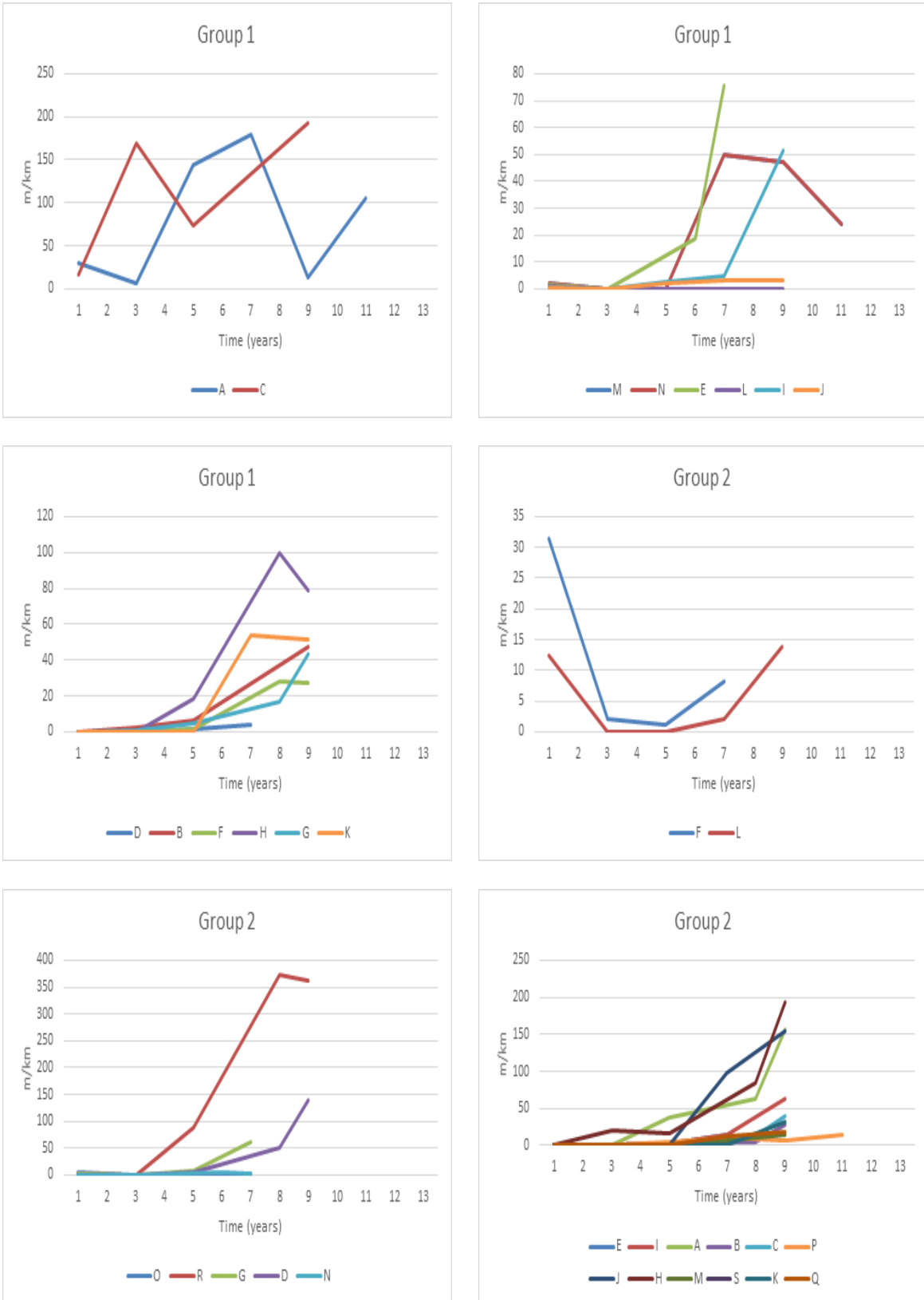
Figure 17. Low longitudinal cracking deterioration on wheelpath for Groups 1 and 2
