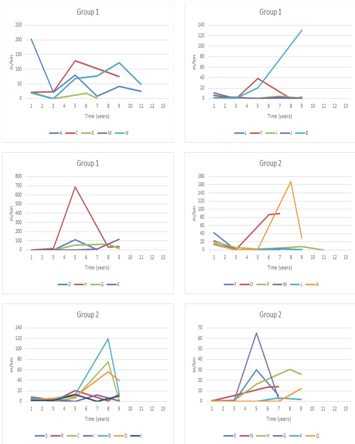
Figure 13. Moderate longitudinal cracking deterioration for Groups 1 and 2
