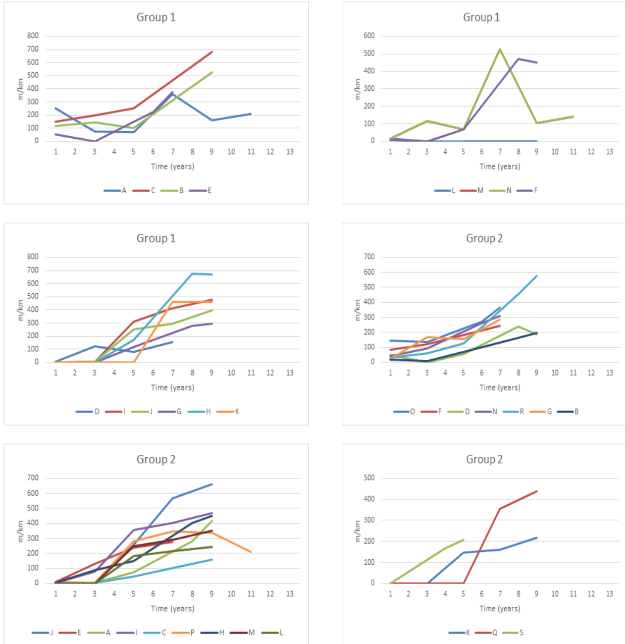
Figure 5. Low transverse cracking deterioration for Groups 1 and 2
