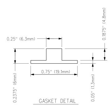
MANHOLE COVER GASKET (SANITARY SEWER)
