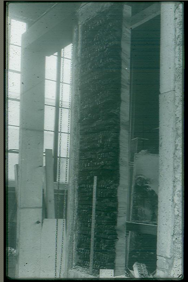
Charred wood slab in FPL wall furnace
