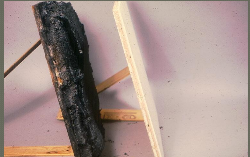
Intumescent coated plywood before and after fire exposure.
