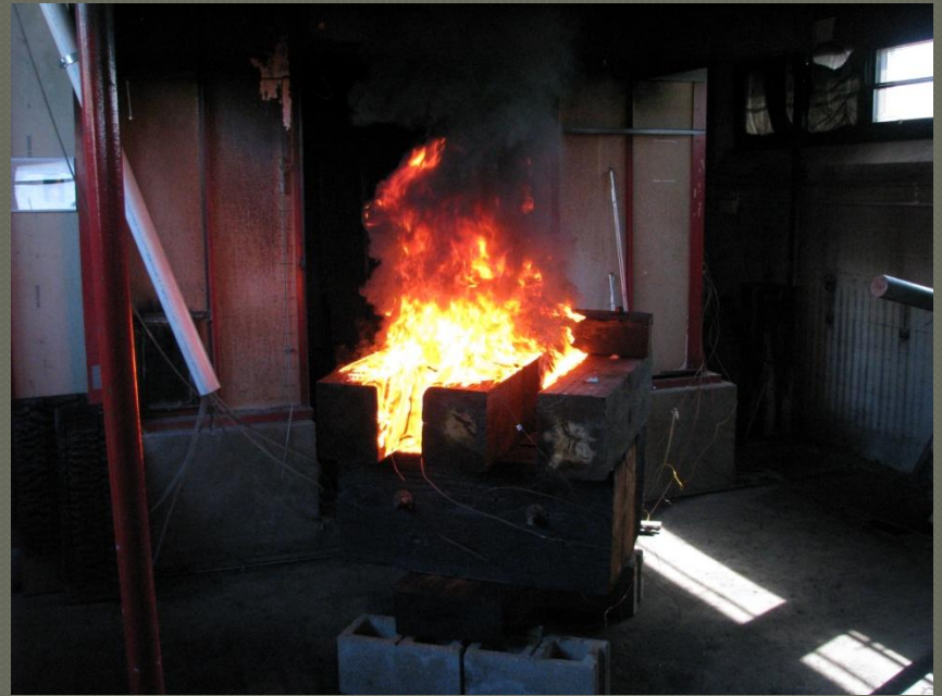
Creosote-treated wood bridge deck crib under fire test hood at FPL
