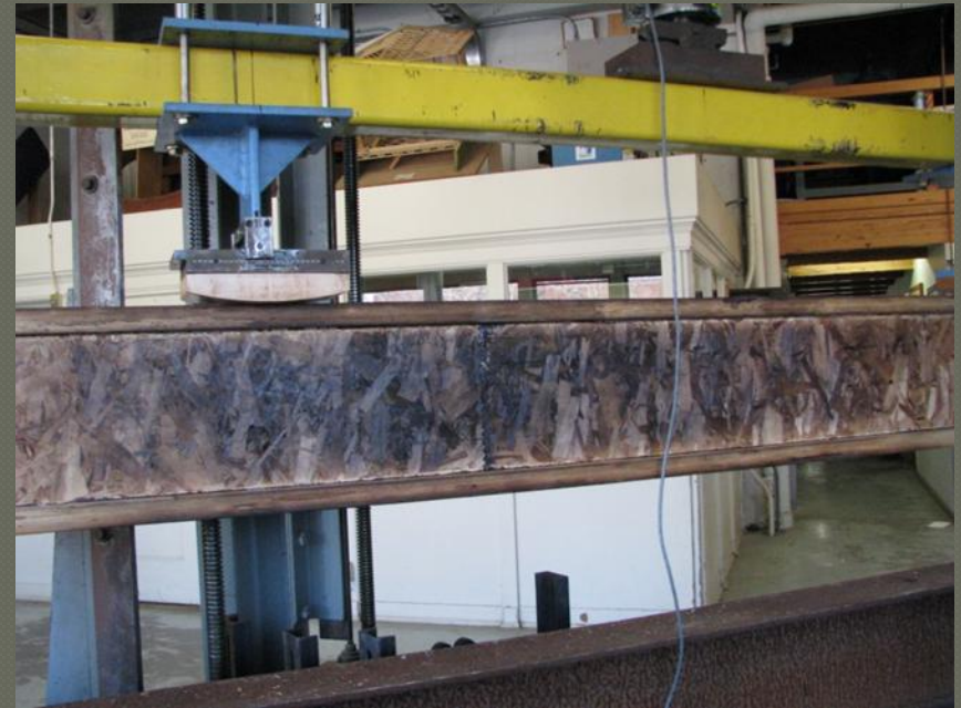
Bending test of slightly charred I-joist.
