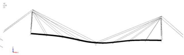
Fig. 6: Vertical mode, f = 1.4 Hz
