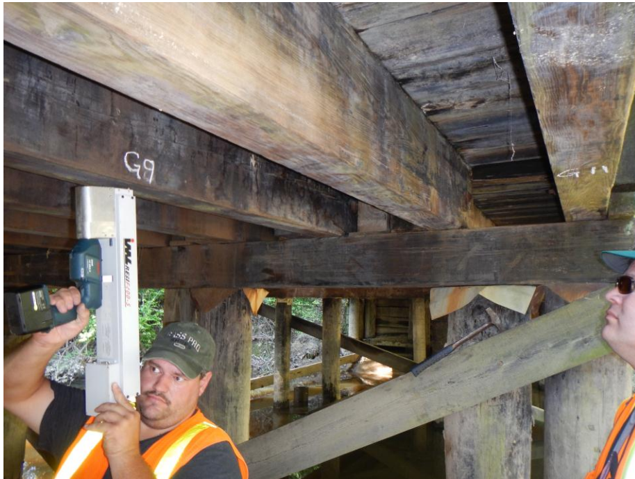
Fig. 5 Resistance Microdrilling to assess condition of stringer
