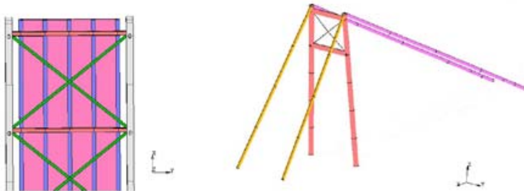
Fig. 6. View from the bottom of the deck (left), and details of the antenna and the tubular oblique elements (right) as implemented in the MSC Marc-Mentat2010 software.
