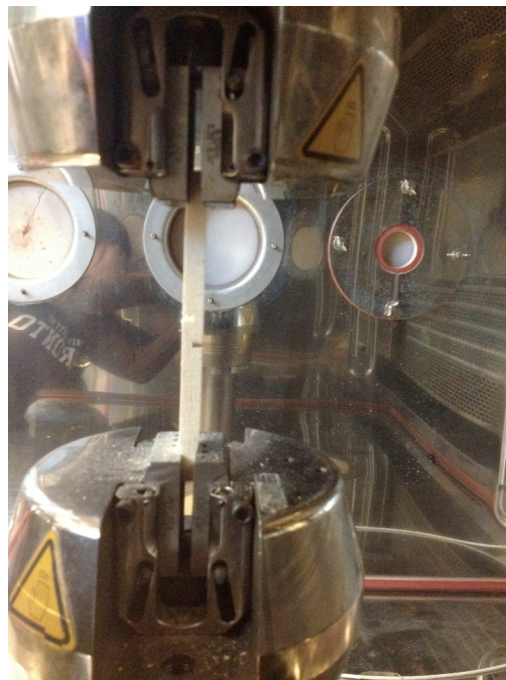
Figure 1. Universal testing machine with wood specimen, in climate chamber.
