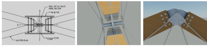
Fig. 10 Connection at the apex of the pyramid frame: engineering drawing, top view and rendering of the elevation,
