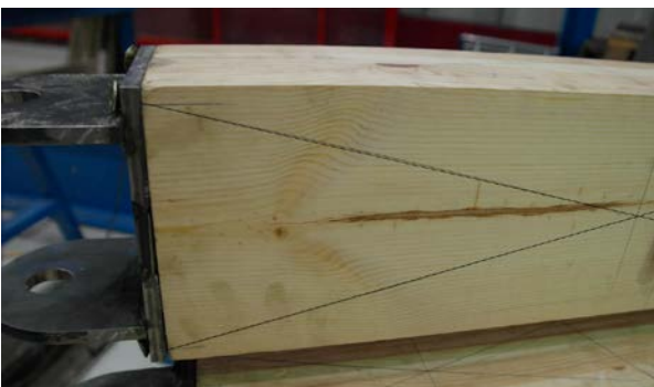
Fig. 12 Support conditions; hinged in the plane of the arch, transversely rigid
