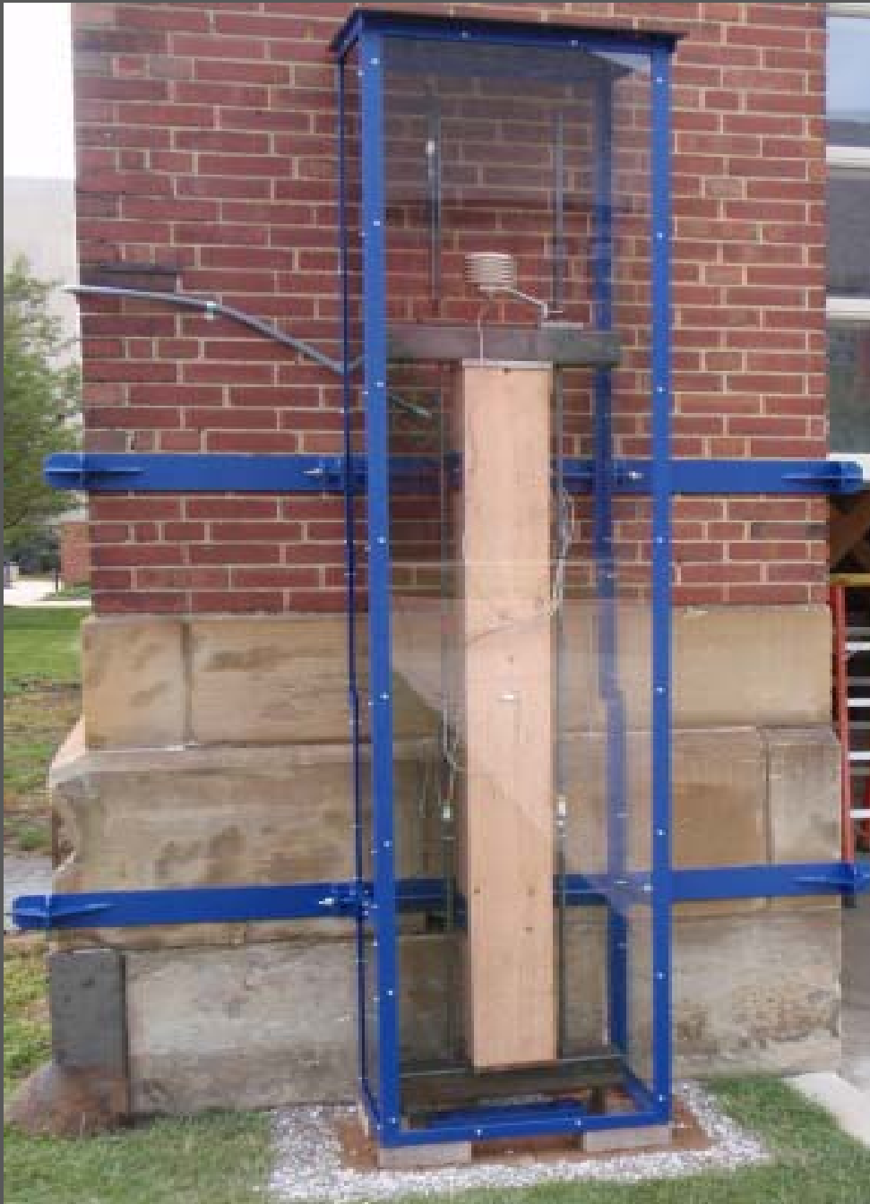
Single 8" x 8" Douglas fir post-tensioned specimen
