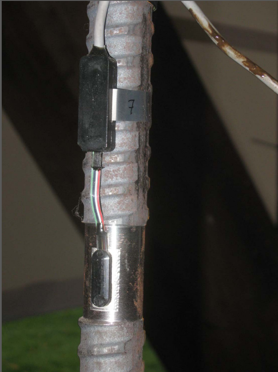
Weldable full bridge strain gauges, HPI model HBWF-35-125-6-10GP-TR-1" PC applied on Diwidag bars
