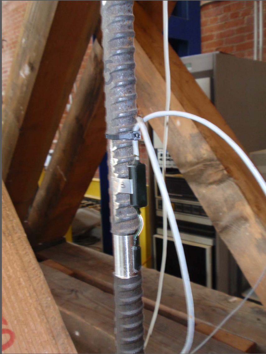
Instrumentation of two Howe trusses
