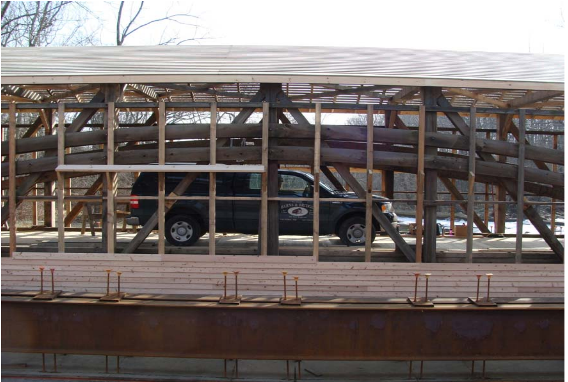
7300 # vehicle, 1/16" deflection recorded by strain gauge
