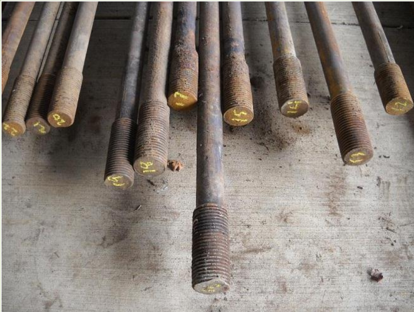
Hanger rods with upset threads
