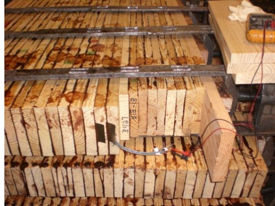
b.) Checking the gages with a volt meter
