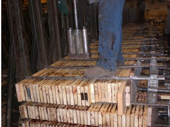
a.) Aligning the laminates in the clamping apparatus
