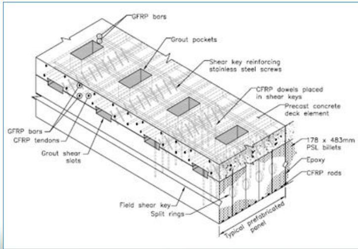
CFRP reinforced PSL/precast concrete configuration
