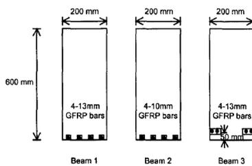
Figure 8 Full-scale specimen cross-sections
