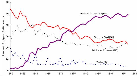
Figure 1 – U.S. New Bridge Material Comparison, 1950-2000
