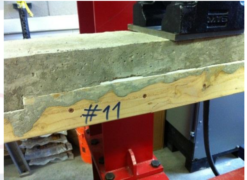
Typical tension failure
