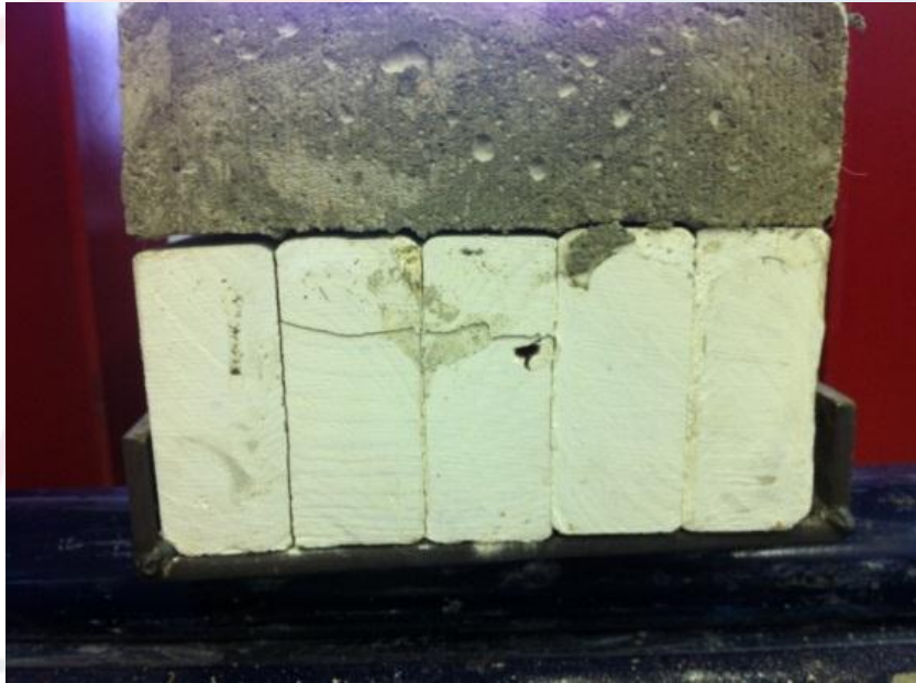
Typical block-shear failure
