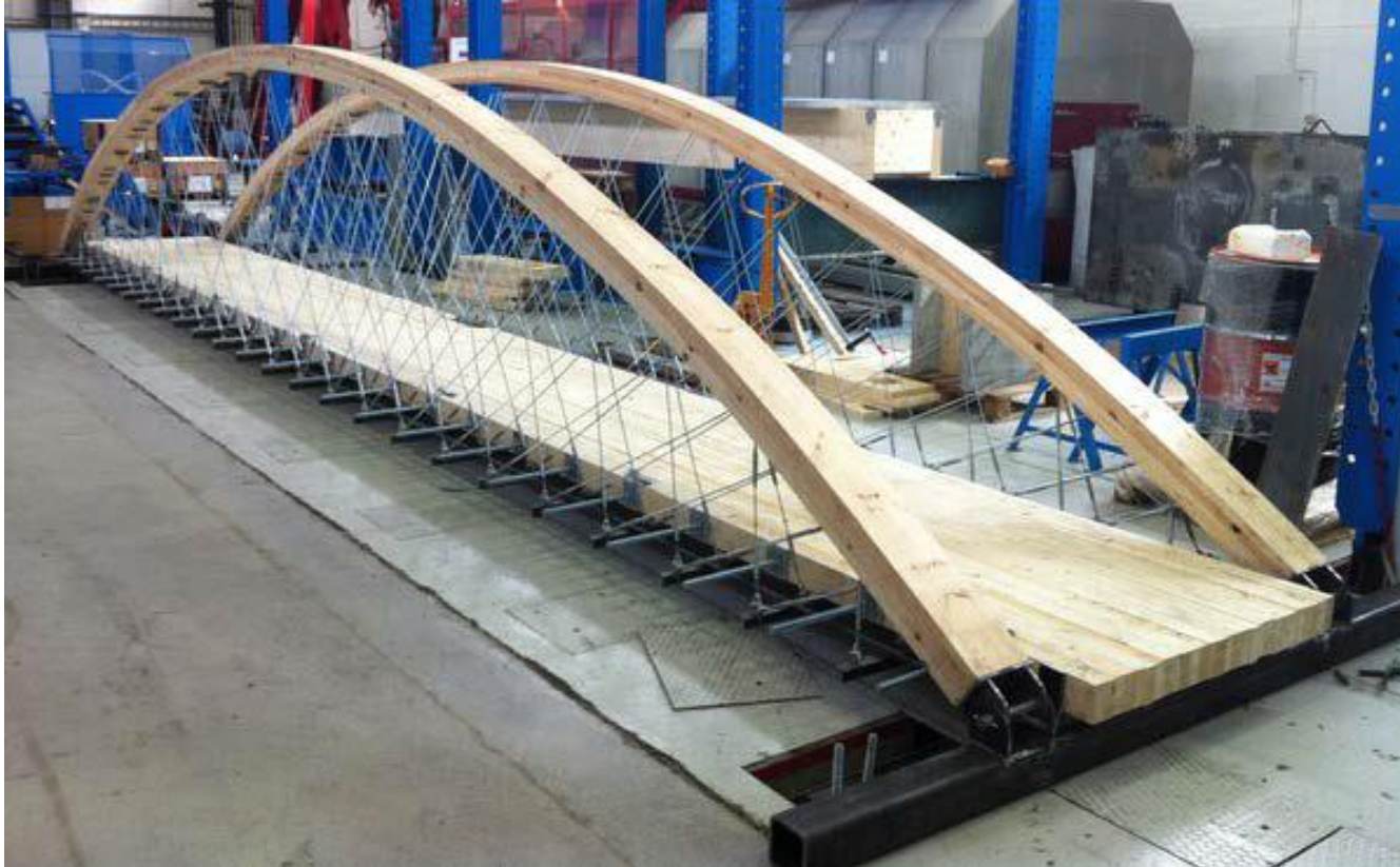
Experimental model in scale 1:10
