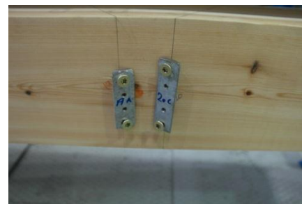
Fastening of hangers to the wooden arch
