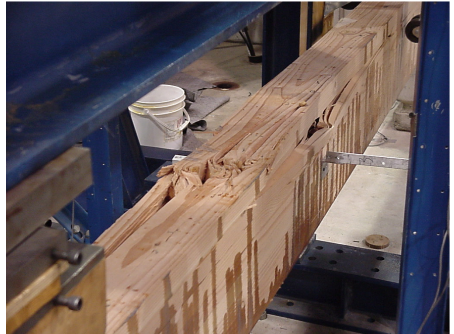
Compression failure (post-fatigue)
