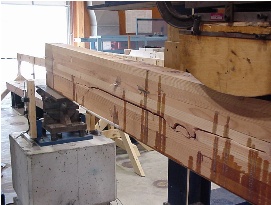
Shear failure (post-fatigue)
