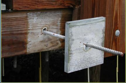
Bridge fastener damage following exposure to water-based preservative
