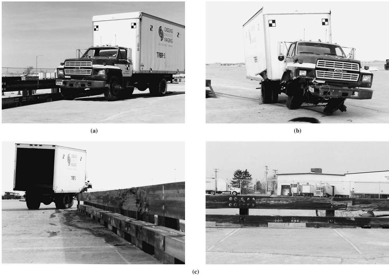
FIGURE 5 Test TRBR-1: (a) impact location, (b) vehicle damage, and (c) bridge railing damage.
