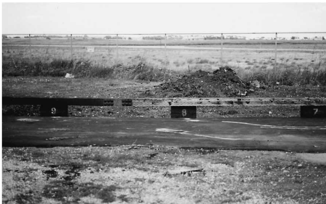
FIGURE 4 Bridge railings successfully crash tested to NCHRP 350 TL-1 (longitudinal deck).
