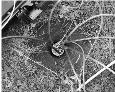
CBST device in borehole ready for test in Ames, Iowa
