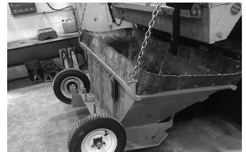
Jones County’s stone placement apparatus
