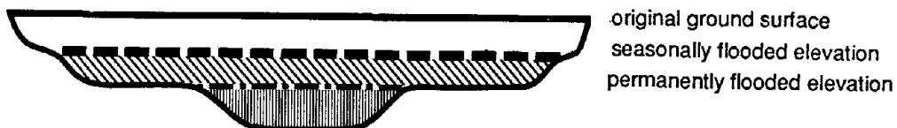
Figure 17. Sizing a wetland basin for significantly expanded seasonal flooding (ground water system).
