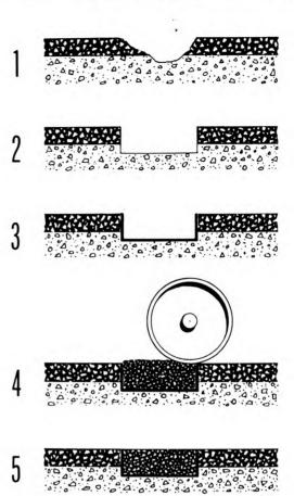
3. Pothole permanent repair. 1) Untreated pothole, 2) Surface and base removed to firm support, 3) Tack coat applied, 4) Fulldepth asphalt mixture placed and being compacted, 5) Finished patch compacted to level of surrounding pavement.
