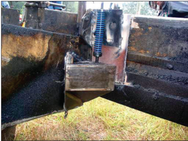
Close-up of safety edge in place on paver (left) and 30° edge slope (right) (photos courtesy of FHWA)
