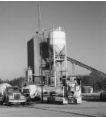
Quality control at the plant is critical to using admixtures and blended cements successfully in concrete mixtures for pavements.
