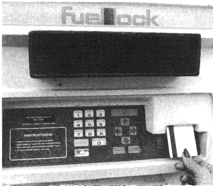
Magnetic cards control access to fuel pumps.
