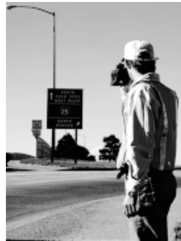
Retroreflectometers help agencies meet new standards for sign and pavement markings retroreflectivity. Photo courtesy of Laser Technology, Inc.
