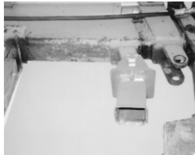
Ray Myers's hydraulic boom-mounted receiver for installing sign posts (perspective is from below the receiver).
