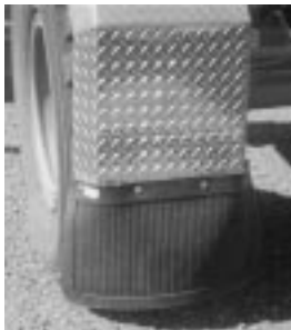
Ageson's motor grader has big, shiny fenders that help protect his windshield and make his motor grader look better. Photos courtesy of Robert Ageson.
