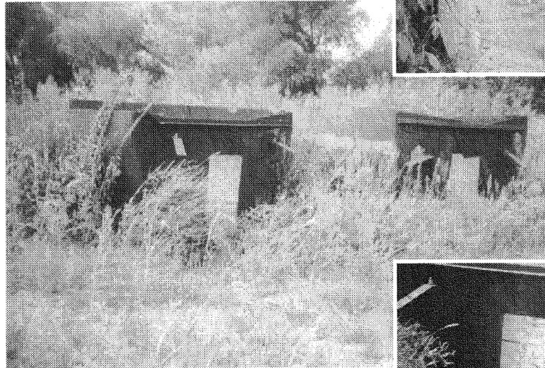
Photo shows two liners. Insets show (top) opening cut for cylinder and (bottom) angle iron attached for running straps to the front of the truck box.
