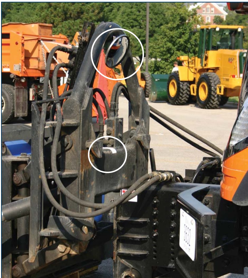
A mirror and some silver tape make it easier for a driver to load a plow alone.
