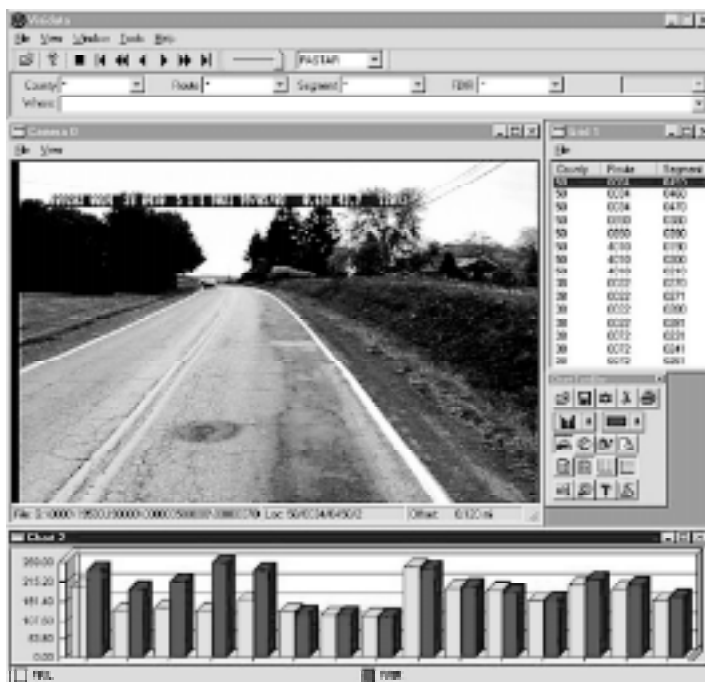
This is an example screen from VISIDATA that shows a front right-of-way view and the pavement condition associated with it (bottom). In the upper right corner, users can scan through the different routes or highways in their network and select the sections they are interested in.
