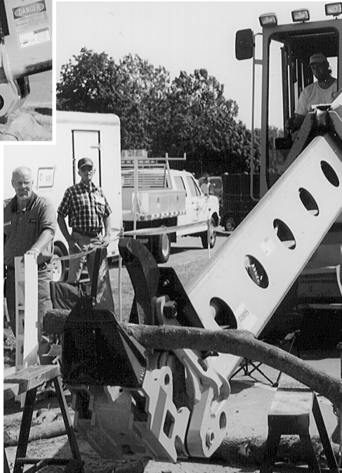
The limb lopper is mounted on a Gradall boom.
