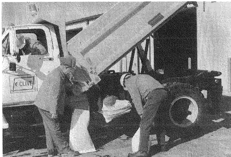
Photo 2 – The truck's design allows the driver to be close enough to the workers filling sandbags to know when to start and stop the device.
