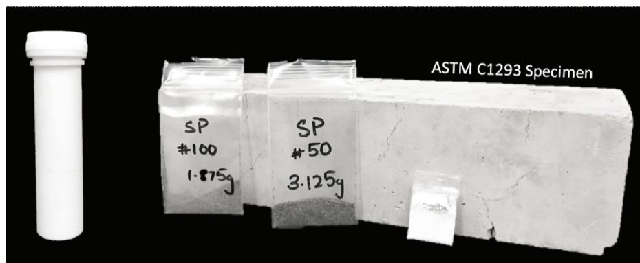
Figure 1. Comparison between the T-FAST test tube setup and a typical concrete prism specified in ASTM C1293
